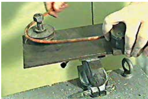
Cable then bent at the point of impact through 180°.
